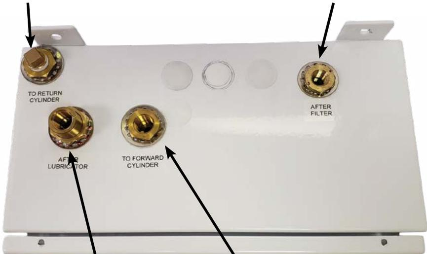
Connect to point after existing airline lubricator.
