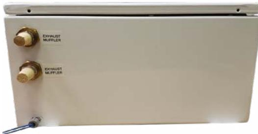
Install two exhaust filters, provided with this system, into the two bottom ports.
