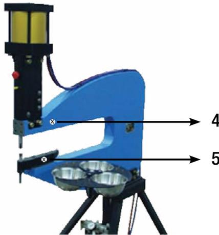
Connect two blue wires from the soft touch enclosure to these two points
