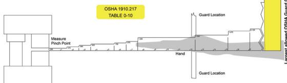
A guard opening scale can be used to measure guard openings and distances from the P.O.O.
