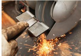
OSHA 29 CFR SubPart O 1910.215 is a “machine specific” (vertical) regulation with a number of requirements, which if left unchecked, are often cited by OSHA as violations. ANSI B11.9-2010 (Grinders) and ANSI B7.1 2000 (Abrasive Wheels) also apply.
