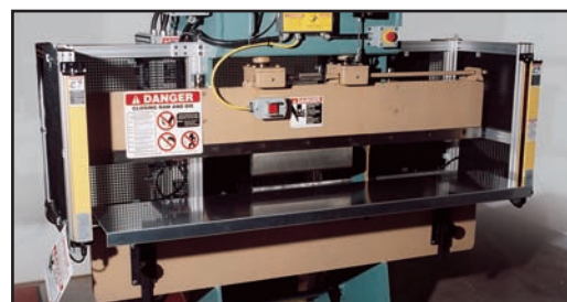
Press Brake With Light Curtain Safeguarding and Clutch/Brake Control
