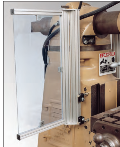
Rear shield assembly on left side of machine column.
