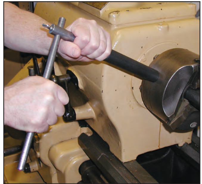
Adjusting the chuck using a long-handled spring-loaded chuck wrench.
