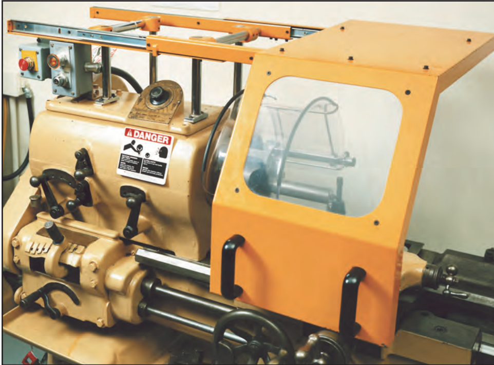
Shield slid into position. Machine is ready for machining workpiece.
