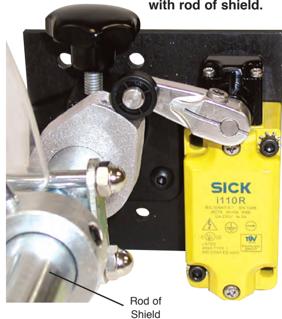
FKT-781 interlocking bracket assembly shown with rod of shield.
