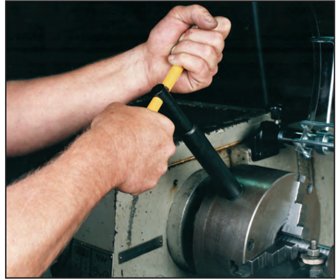
Adjusting the chuck using a spring-loaded chuck wrench.
