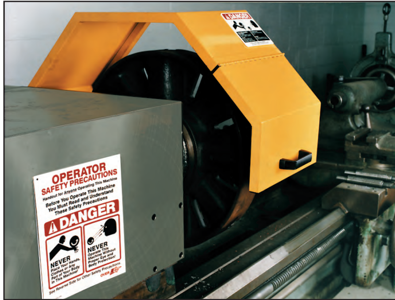
The hinged portion can be swung up for workpiece changes.
