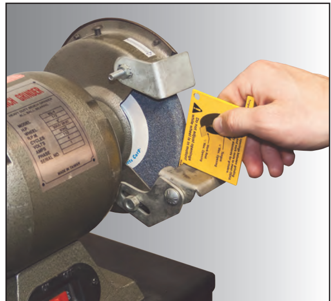
Checking work rest opening.
