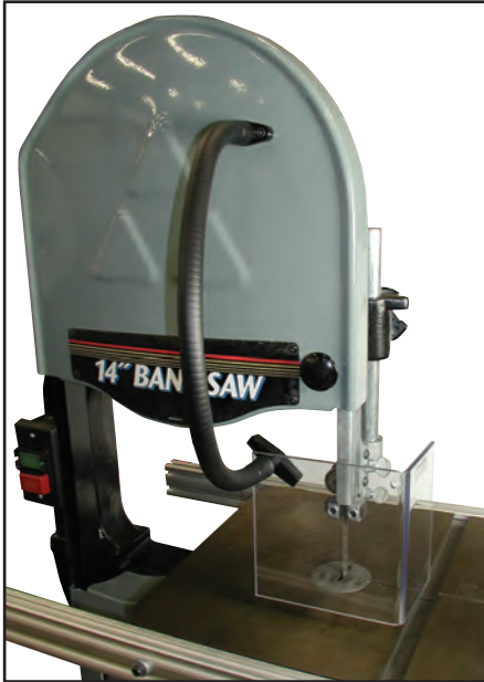
Flexible spring-steel arm band saw shield.
