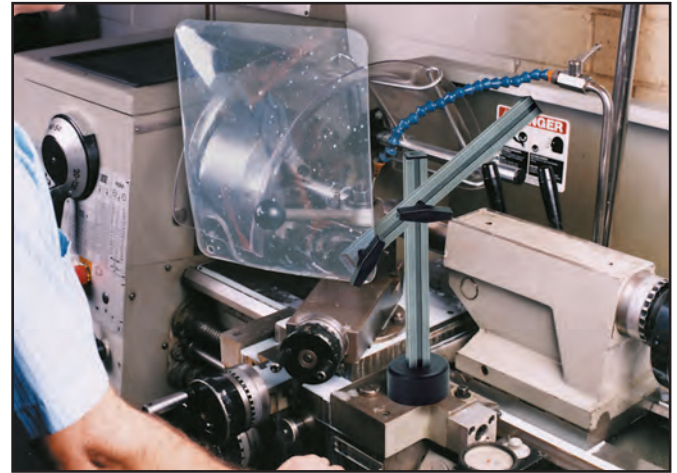
Magnetic-base concave shield shown on a lathe.
