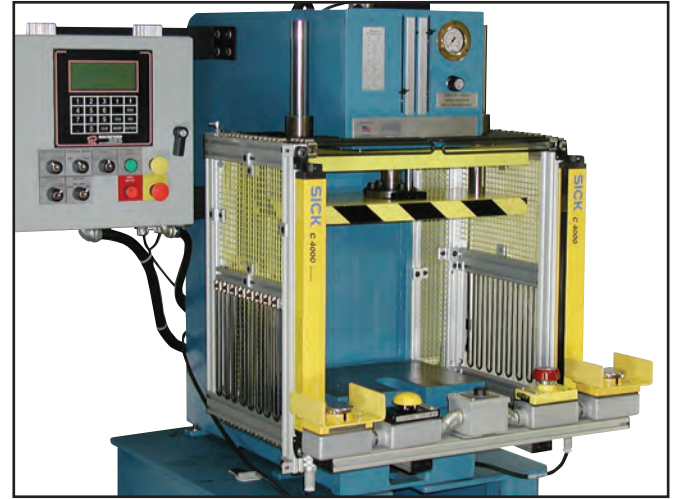
Hydraulic press with a light curtain and two-hand control as the point-of-operation safeguard.
