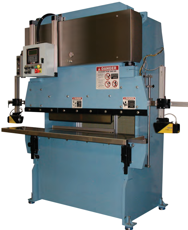
Hydraulic press brake with V4000 safeguarding system.
