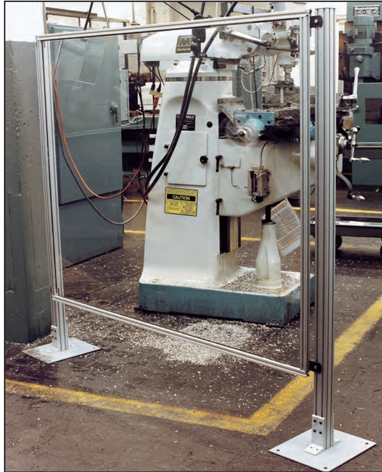
Free-standing shield used to protect the area around a milling machine from flying chips.
