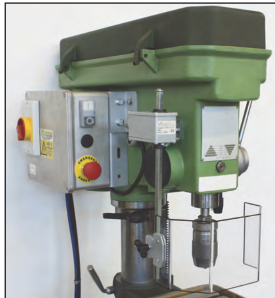
Electrically interlocked shield for small to medium size drill presses.
