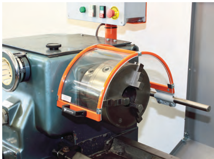
Electrically interlocked chuck shield on lathe.
