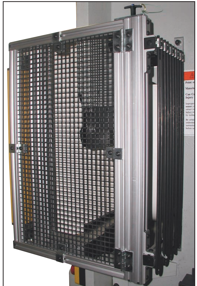
Swing-Away Light Curtain Mounting Bracket With Nonadjustable Guards for Press Brakes
